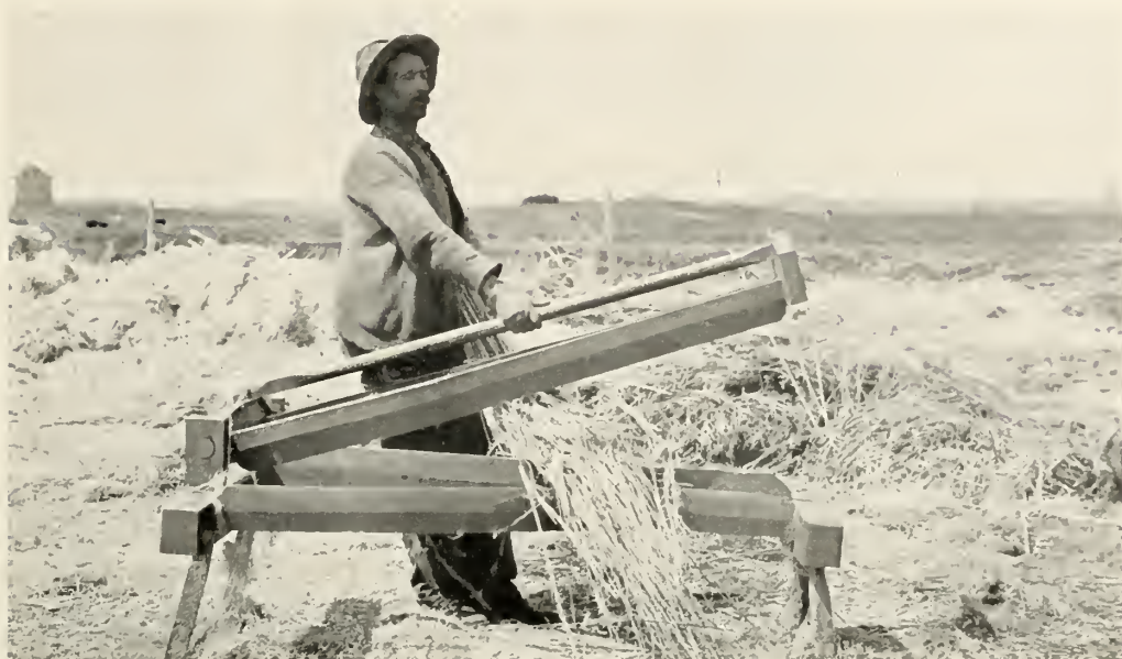
FIGURE 56.—Hand brake by means of which retted hemp stalks are crushed and the woody interior portion broken into small pieces that are removed by whipping the fiber across the top of the brake. Kouts, Ind.
