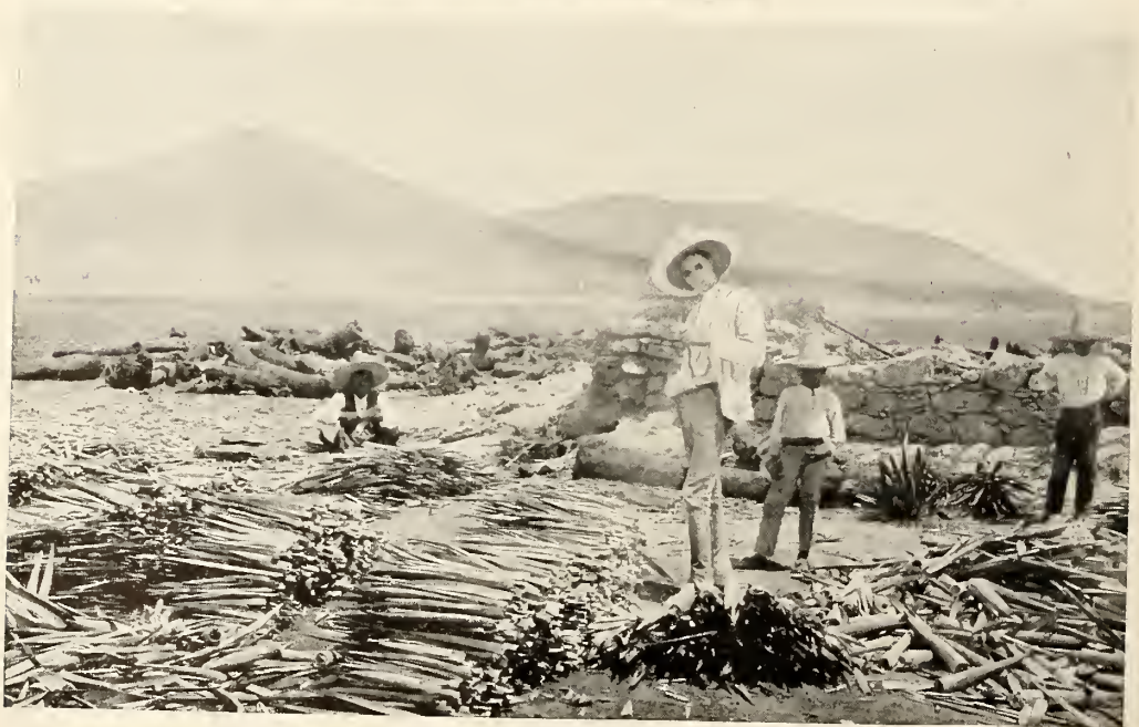
FIGURE 40.—Palma barreta fiber production; plants abundant on hills in background; trunks of palma barreta for burning in the crude stone furnace to steam the cogollos, at right, which are separated into fiber-yielding leaves, in center; these leaves are drawn under a knife by the man sitting on the ground. Carneros Pass, Mexico.
