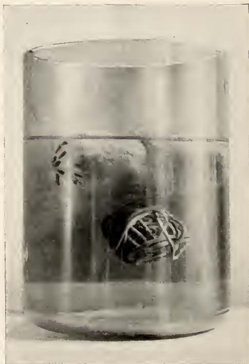
FIGURE 70.—Buoyancy test of northern pochote fiber. Ten grams of fiber, in a cheesecloth sack carrying a weight of 150 gm., beginning to sink at the end of 259 days. Fiber from Sonora, Mexico.
