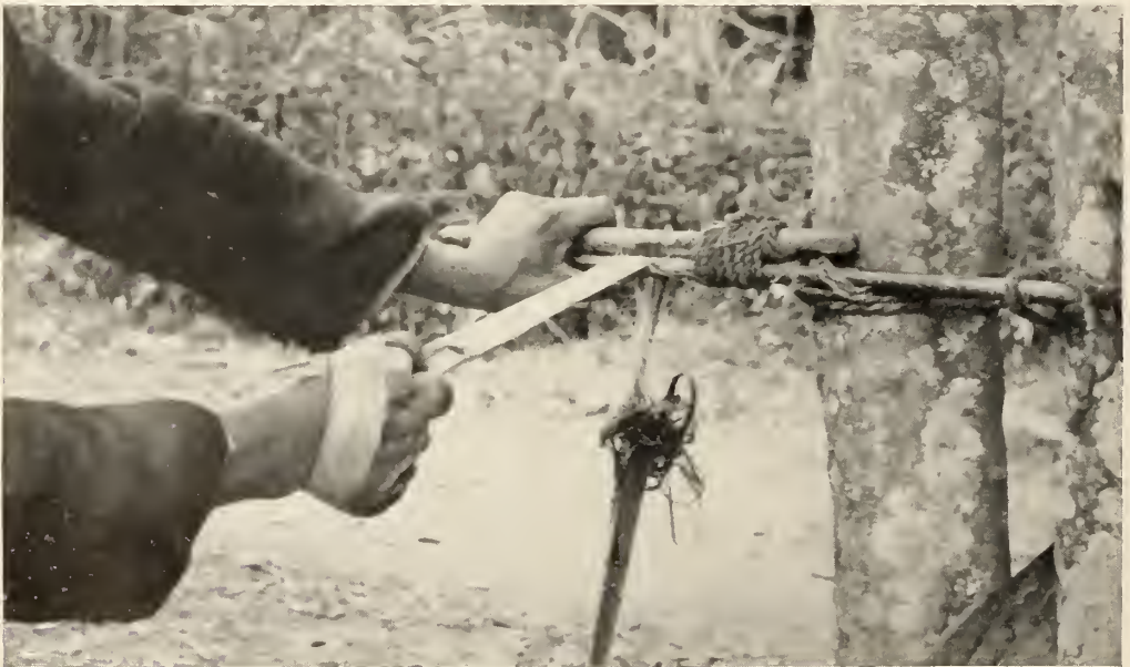
FIGURE 31.—The carrizo. Strips of fique leaves are drawn between two sticks pressed together to scrape away the pulp. Photograph from Sr. Adel López Gómez, of the Ministry of National Economy of Colombia.
